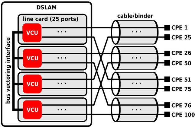
Fig. 2: Topology of simulated VDSL2 deployment scenarios
