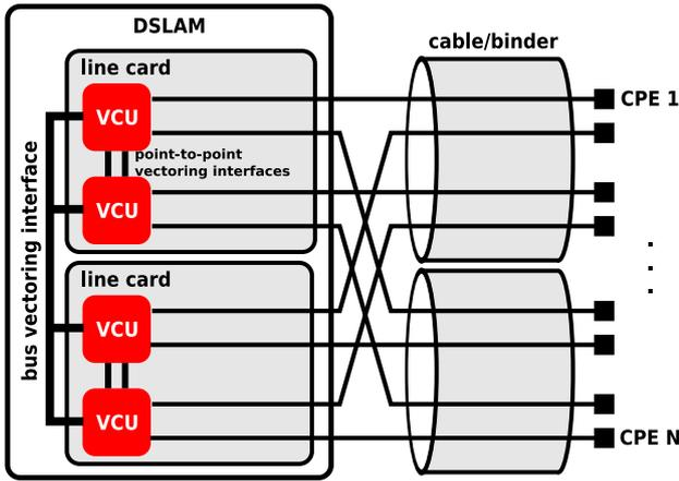
Fig. 1: xDSL scenario with restricted signal-level access of VCUs to lines.
